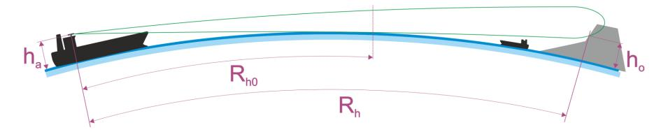
the ability to detect objects, beyond the horizon, depends on the height of the antenna and the height of the detected object. This corresponds to the formula:
