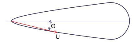
Directional antenna: the intensity of radiations U changes as a function of the angle  $\Theta$ . maximum value of the intensity occurs, when  $\Theta=0$ ;
