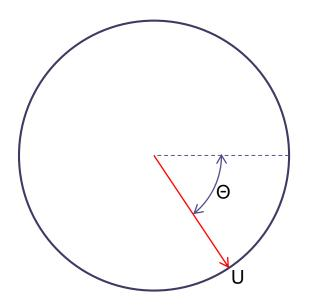
Isotropic antenna: the intensity of radiation is independent to the angle  $\Theta$
