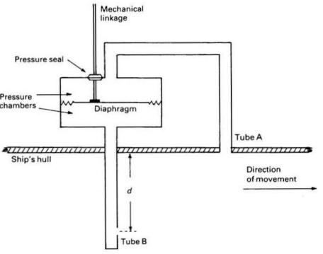
As the vessel moves through the water, in the direction shown, water is forced into tube B producing a combined pressure in the lower half of the chamber equal to both the static and dynamic pressures. The difference in pressure, between upper and lower chambers, now forces the diaphragm upwards thus operating the mechanical linkage. Obviously the greater the speed of the vessel through the water, the more the diaphragm will move and the greater will be the speed indicated.
