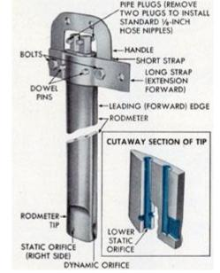
The total pressure in the tube, called a Pitot tube, is therefore the sum of both the static and dynamic pressures. To ensure that the dynamic pressure reading, and thus speed, is accurate, the effect of static pressure must be eliminated. This is achieved by installing a second tube close to the first in such a way that the static pressure produced in it is identical to that created in the Pitot tube but without the pressure increase due to movement through the water.
