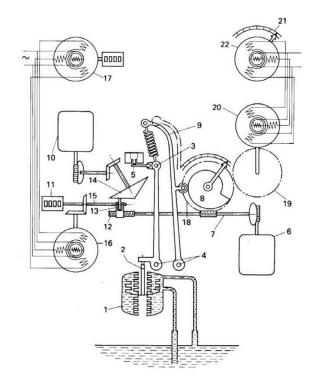
The distance indicator (11) is driven from the constant speed motor (10) via the cone. The nearer to the rim of the cone the friction wheel rides, the greater will be the distance indication. Revolutions of the distance shaft (15) are transmitted to the remote distance indicator via the servo transmission system (16 and 17).
