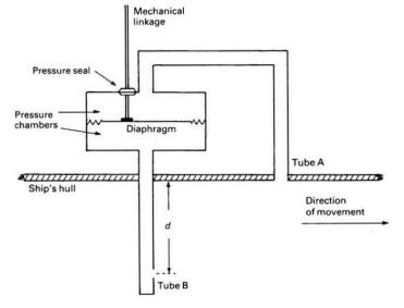
The dynamic pressure developed in tube B, by the relative movement through the water, is proportional to the square of the vessel's speed. Pitot's Law states that this pressure p is proportional to the square of the ship's speed v multiplied by the coefficient K.
