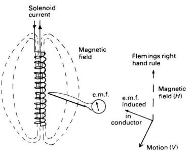
Because  $\beta$  is approximately equal to H (the magnetic field strength), e.m.f. = Hlv assuming no circuit losses.
