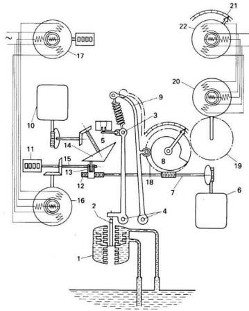
Distance recording is achieved by using a constant speed motor (10) which drives the distance counter (11), via friction gearing. The constant speed motor has been used in order that a distance indication may be produced that is independent of the non-linear characteristic of the system. The motor is started by contact (5) as previously described. The main shaft (7), whose angle of rotation is directly proportional to the speed of the ship, is fitted with a screw spindle (12).
