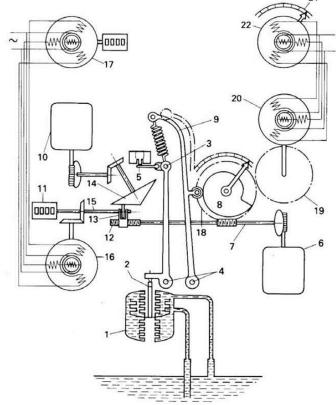
This method of pressure compensation provides accurate indications of speed independent of alterations of the diaphragm caused by ageing. The shape of the spiral cam (8) has been carefully calculated to produce a linear indication of speed from the non-linear characteristics of the system.
