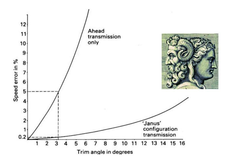
The addition of a second transducer assembly set at right angles to the first one, enables dual axis speed to be indicated
