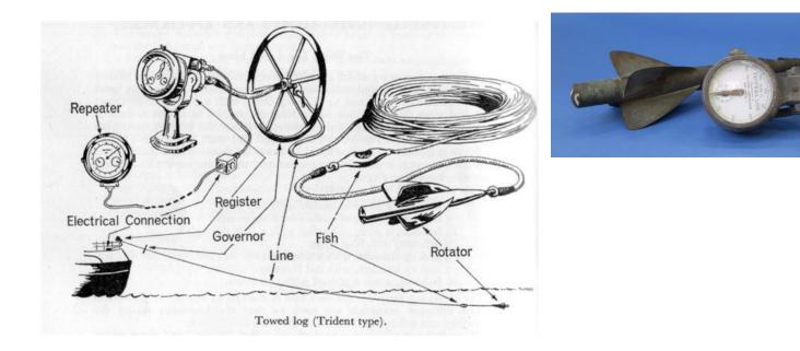
Mechanical logs – impeller log
