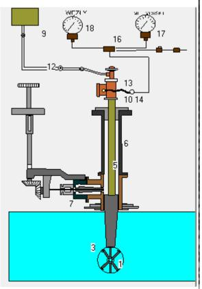
When a tube, with an opening at its base, is vertically submerged in water, a pressure, proportional to the depth to which the tube is submerged, will be developed in the tube. If the tube is held stationary the pressure remains constant and is termed 'static' pressure. If the tube is now moved through the water, whilst keeping the depth to which it is submerged constant, a second pressure called 'dynamic' pressure is developed.
