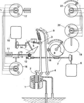
The deflection stretches the main spring, producing a downward pressure on the diaphragm, via lever (3), causing it to cease rising at an intermediate position. This is achieved when equilibrium has been established between the dynamic pressure, acting on the lower side of the diaphragm, and the counter pressure from the spring on the upper side. At this point the motor (6) stops and thus holds the spiral cam (8) in a fixed position indicating speed.
