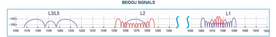
SPECTRAL CHARACTERISTICS OF BEIDOU NAVIGATION SIGNALS
