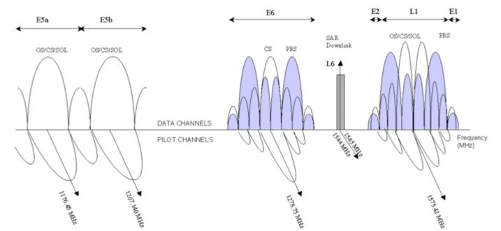
Each Galileo satellite will broadcast 10 different navigation signals making it possible for Galileo to offer the open (OS), safety-of-life (SOL), commercial (CS) and public regulated services (PRS)
